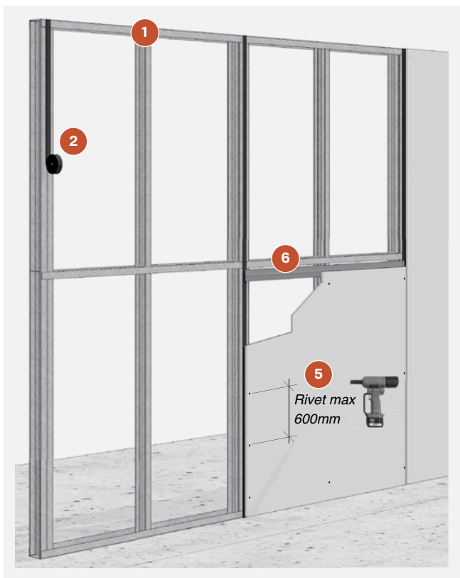
FIGURE 7.29 Concealed Fixing on Steel Frame
